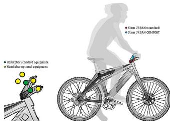
For the ST3, in addition to the Sport and Comfort frame in various sizes we have also developed two different stems (Urban and Urban Comfort) and three different handlebars. You can freely combine these components so that you can enjoy the unique Stromer riding experience in a sitting position that is perfect for your body size.
